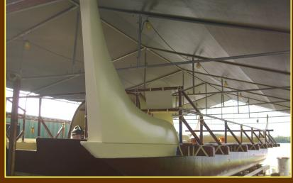
The Moku Kaha`i is a double-hulled flat bottom boat that is inspired by the design of the Hōkūle`a (a replica of an ancient Polynesian double hulled voyaging canoe)
